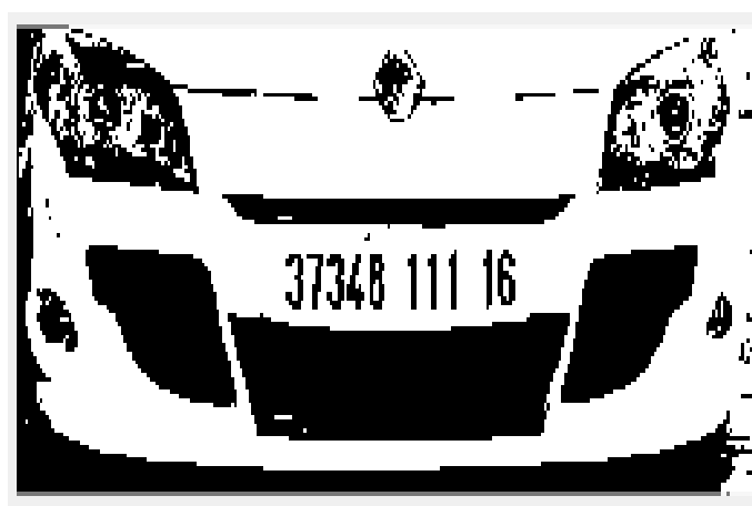
Figure 2.4 Binary Image Using Otsu's Method.
